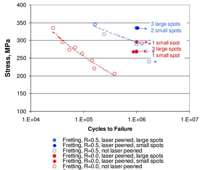
Figure 7. Increased fretting fatigue life after laser peening of Ti-6Al-4V.
