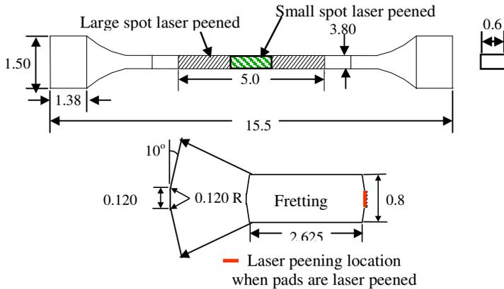
Figure 4. Fretting fatigue specimens and pads showing the laser peened areas. Dimensions are in inches.
