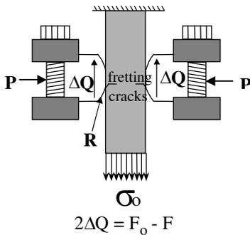
Figure 5. Schematic of the fretting fatigue test set up, from [3].
