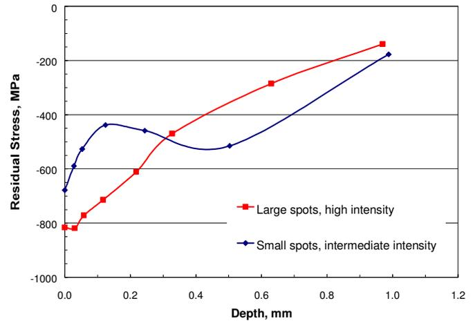
Figure 6. Residual stress profiles for the large spot and small spot laser peening conditions used for the fretting fatigue tests.
