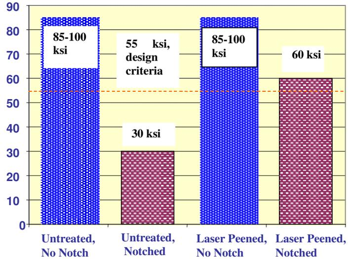
Figure 3. The effect of laser peening on F119 IBR fatigue life. A 0.050-inches deep EDM notch was used on the notched airfoils.
