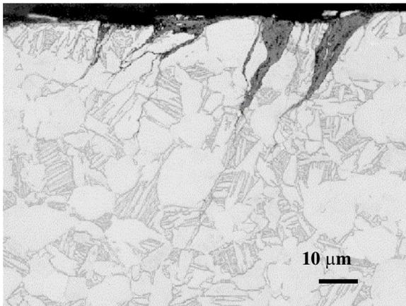
Figure 8. Fretting cracks at the trailing edge of the contact surface on fretting fatigue bar tested to runout at fretting fatigue stress level S2.
