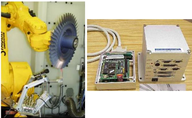
Figure 1. RapidCoater™ system set up for processing an F119 Integrally Bladed Rotor (left) with a dedicated computerized control module (right).
