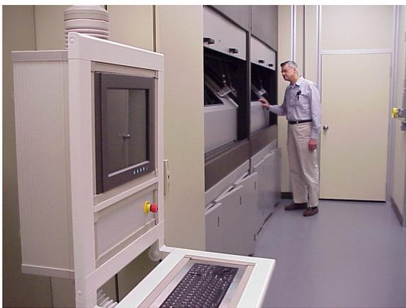
Figure 2. ManTech laser peening system featuring high rate processing with robust, production hardened equipment.
