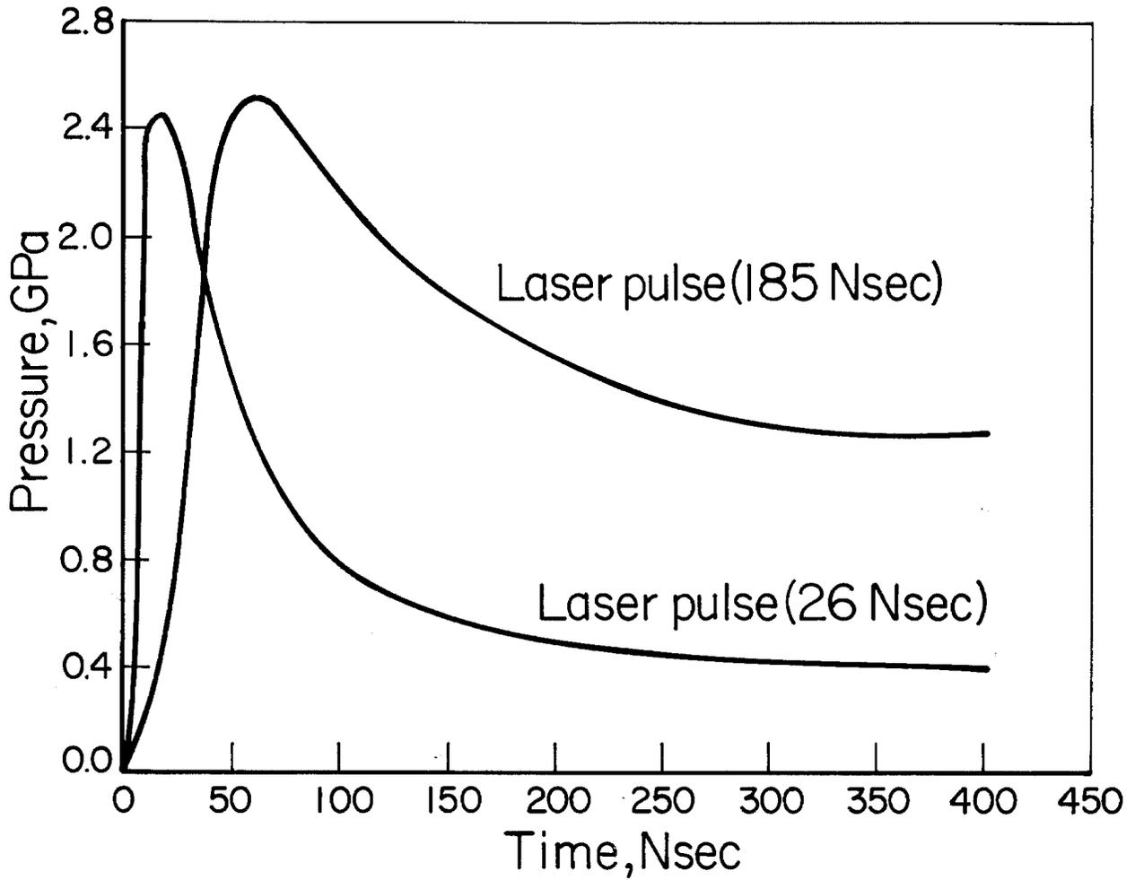
Fig. 2. Comparison of pressure pulses generated by different laser pulses, Pressures measured through  $1.27 \times 10^{-3}$  cm thick Zn foils covered with 0.3 cm thick quartz discs.
