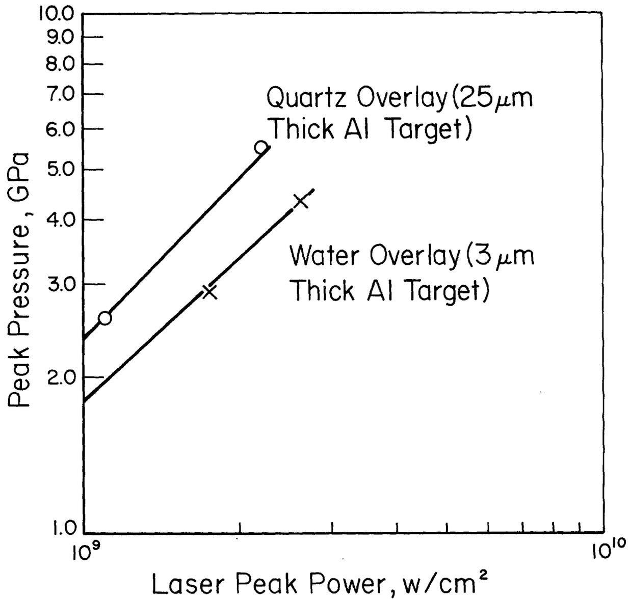
Fig. 1. Peak pressures measured through thin aluminum targets. Lines through the data represent extrapolations of published results at lower laser peak powers.
