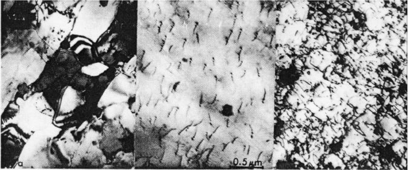
Fig. 5. Microstructure of 5086 H32 aluminum sheet before and after welding and laser shocking. (a) Initial condition - 5086 H 32, (b) After welding - in the heat-affected zone adjacent to the weld zone, and (c) After laser shocking - in the heat-affected zone adjacent to the weld zone.
