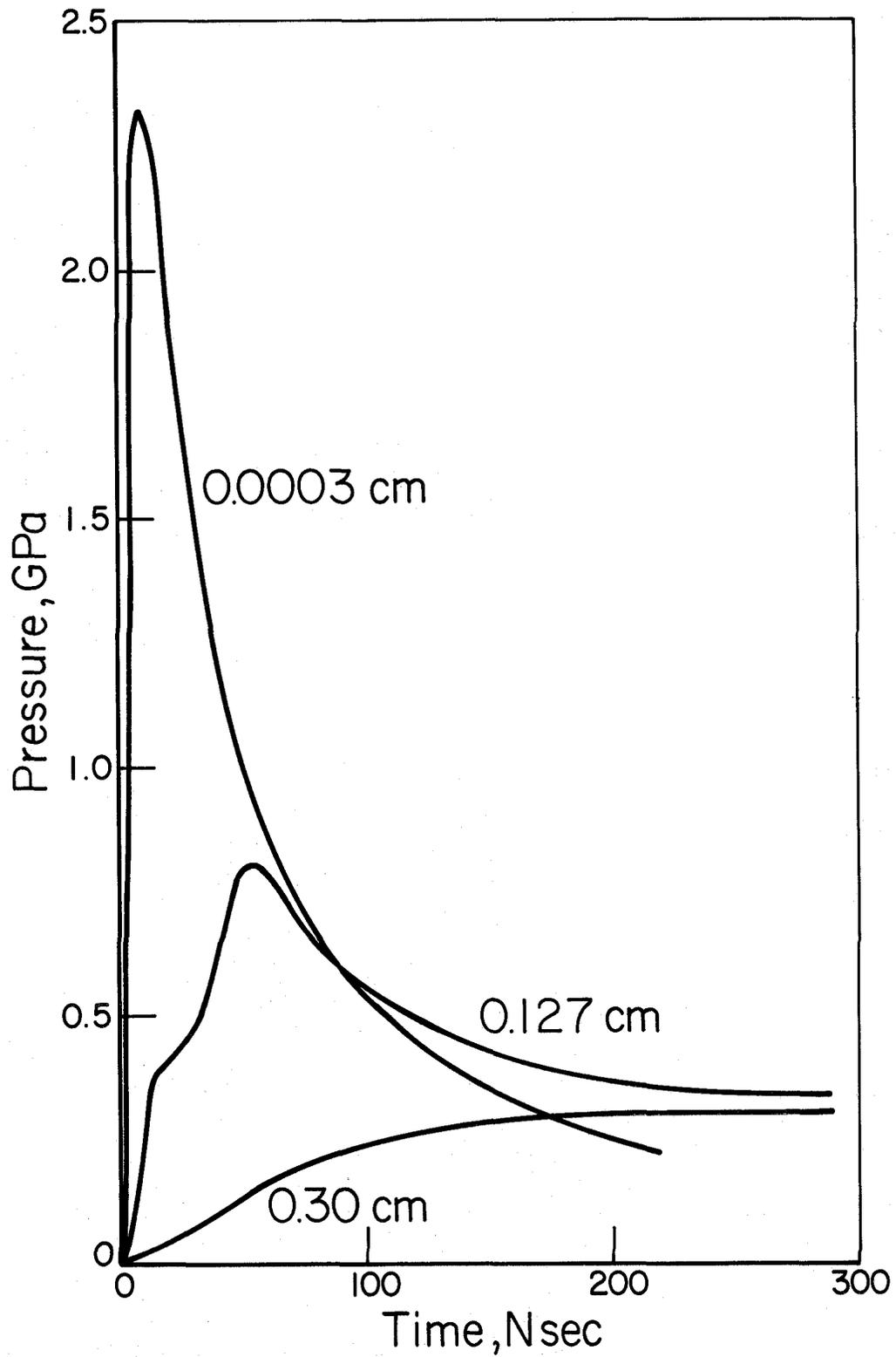
Fig. 4. Pressure pulse in aluminum for various penetration distances (Water overlay).
