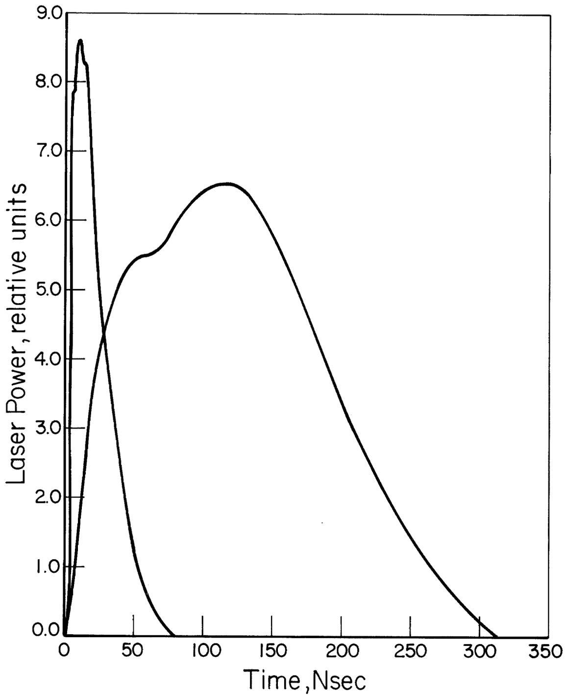
Fig. 3. Comparison of laser pulses used in pressure generation.
